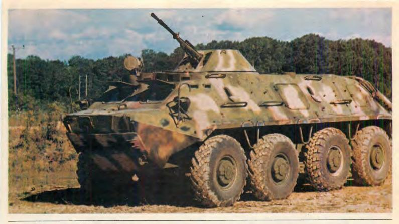
Above: BTR 60 showing 14.5mm main gun; shield just below bow of vehicle is raised when going through water to prevent splash. Photo credit: U.S. Army.
